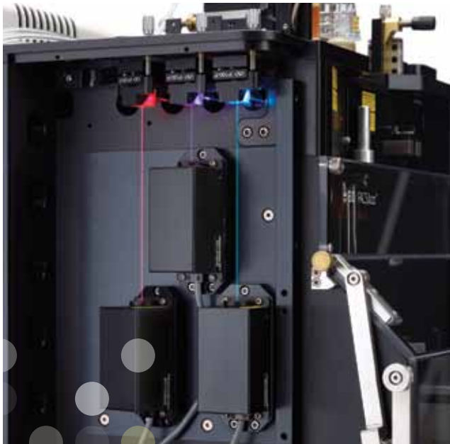
Inside view of lasers and laser steering module
